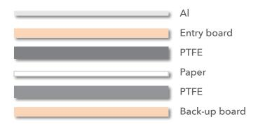
For hybrid multilayers combined with PTFE and FR-4, drilling is recommended to put PTFE at the bottom and FR-4 on the surface.
